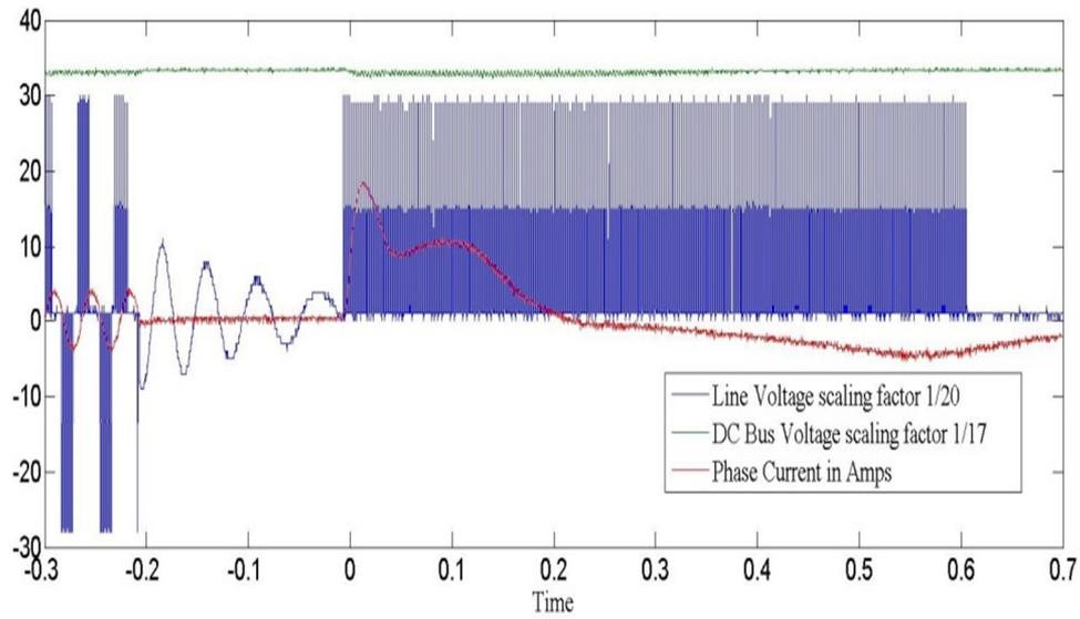
**Figure 10.** Line voltage, stator current and Bus voltage when applied advance D.C. Injection Braking
