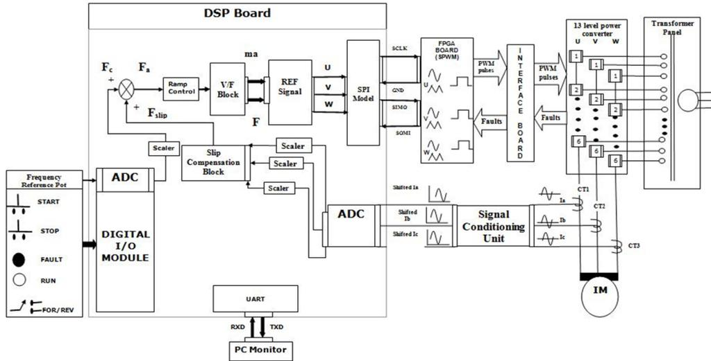
Figure 9. Control Block diagram of complete system
