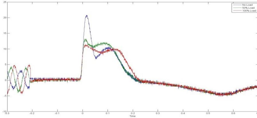
**Figure 13.** Stator current when applied advance D.C. Injection Braking at 500 rpm
