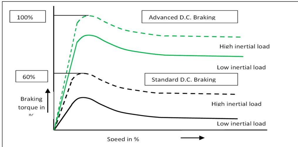
**Figure 3.** Torque Speed Curve of IM
