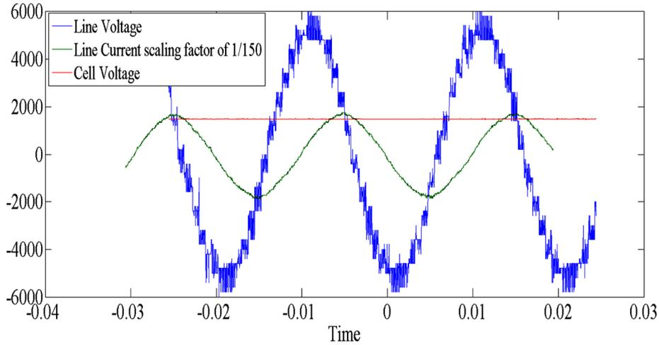
Figure 5. Output voltage, current and cell voltage waveform for 13 level inverter
