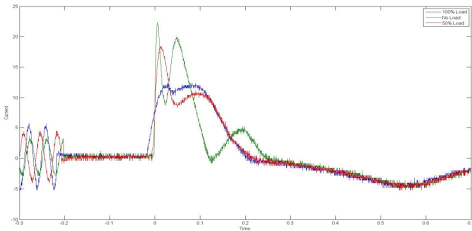
**Figure 12.** Stator current when applied advance D.C. Injection Braking at 800 rpm
