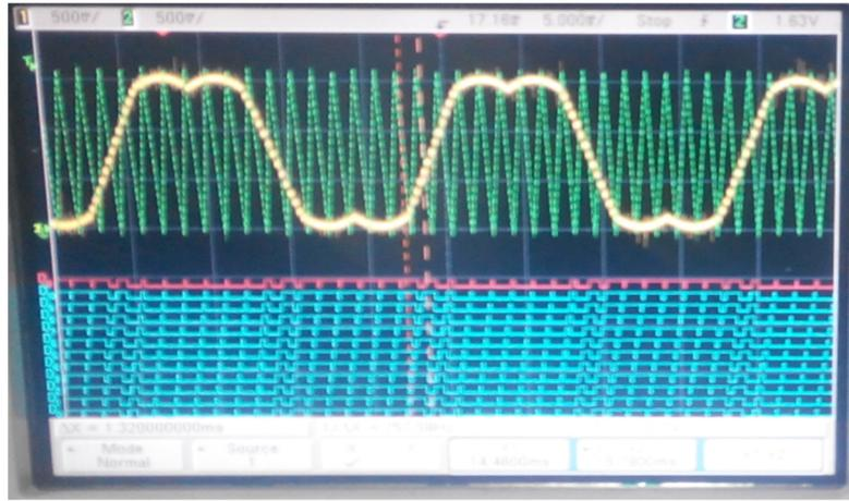
**Figure 1.** Modulating signal, carrier wave and 12 PWMs for single leg
