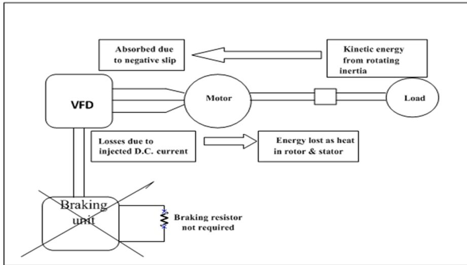
Figure 6. Balance of energy during D.C. braking
