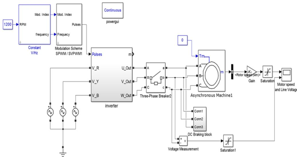
Figure 7. MATLAB circuit of D.C. injection braking
