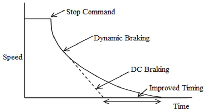
**Figure 4.** Stopping with dynamic braking and D.C. injection braking
