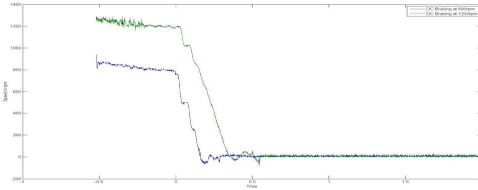
**Figure 14.** Speed-time curves when D.C. Braking applied at 1200rpm and 800rpm
