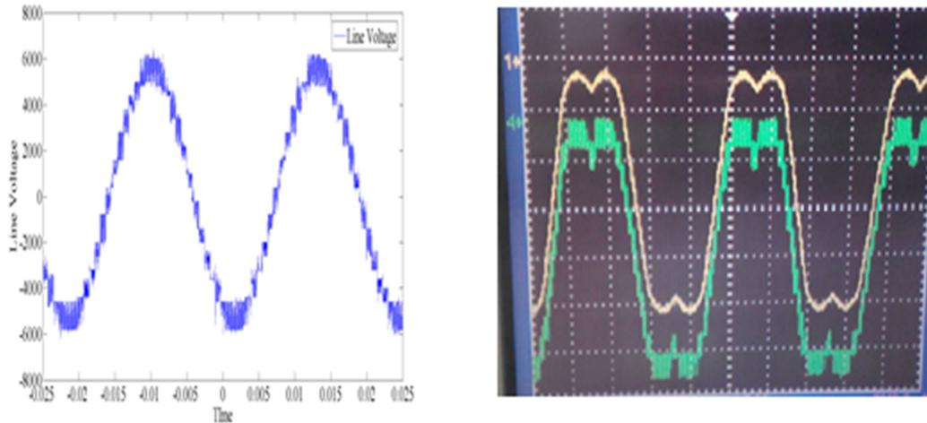
**Figure 2.** 13 level line-to-line multilevel voltage and phase to neutral voltage
