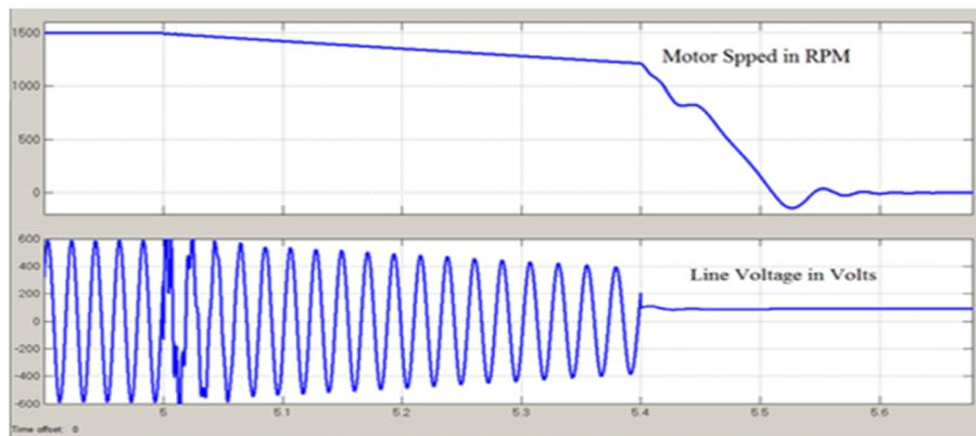
Figure 8. Speed-time curve and line to line voltage when DC braking is applied
