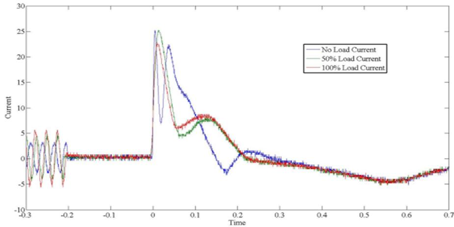
**Figure 11.** Stator current when applied advance D.C. Injection Braking at 1200 rpm
